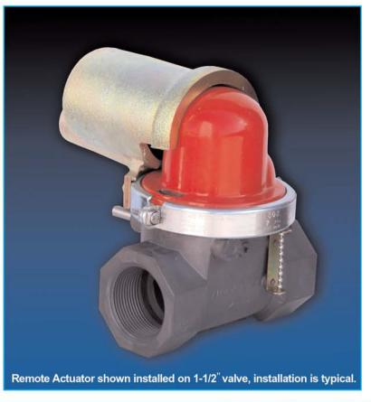
The Model 501 Remote Actuator will add an additional layer of protection to panic switches, fire and sprinkler alarm systems. A CALIFORNIA valve with the 501 Remote Actuator will trip during a violent earthquake or when an electrical signal is present.
